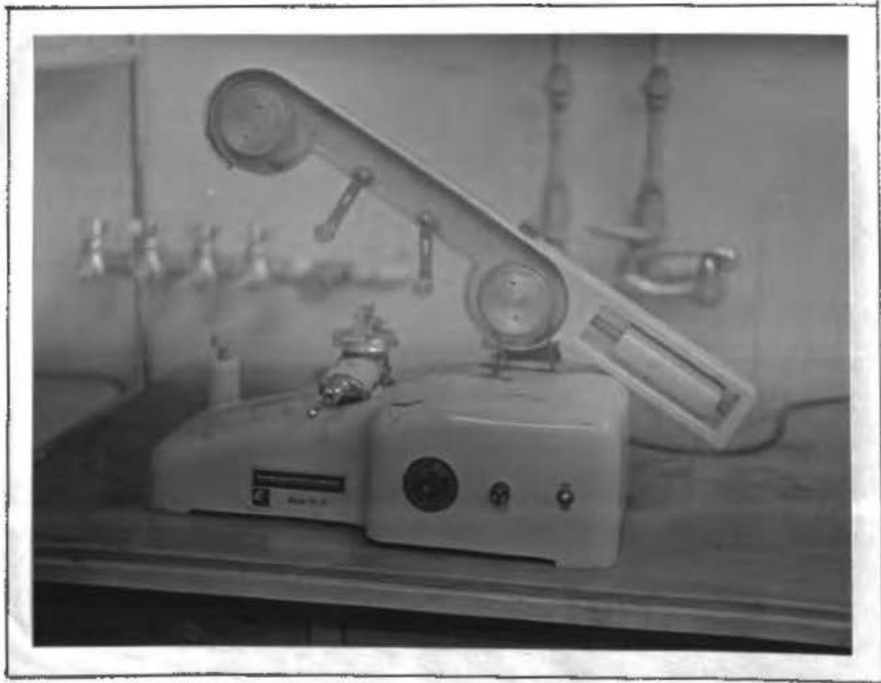
Figure 34. Equipment for cutting wire saw notch into the specimen
