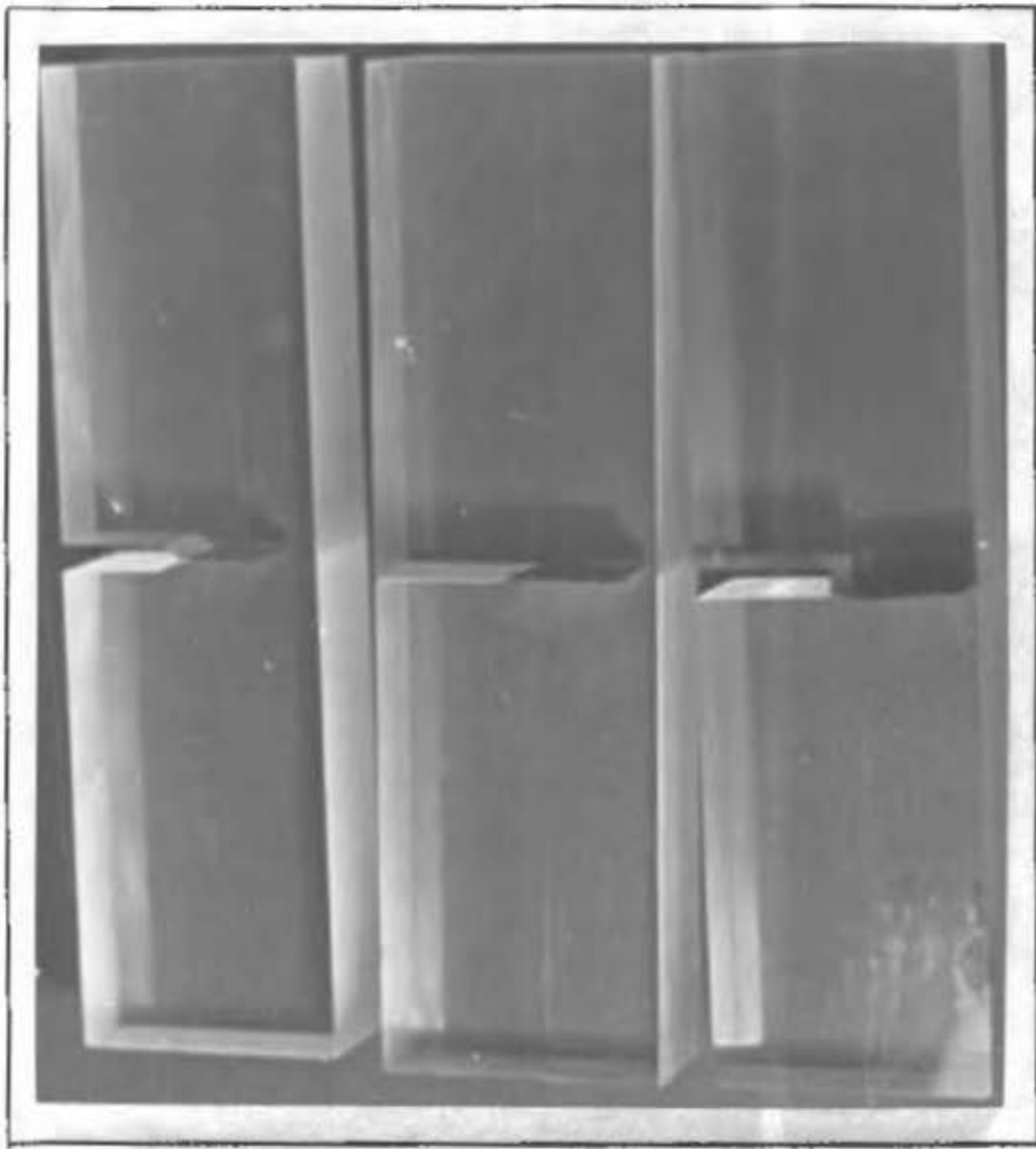
Figure 33. Crack growth for different notch shapes
